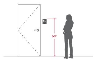
Mounting signage at 60 inches from the top of the sign to finish floor will ensure compliance for any permanent sign less than one foot in height.
